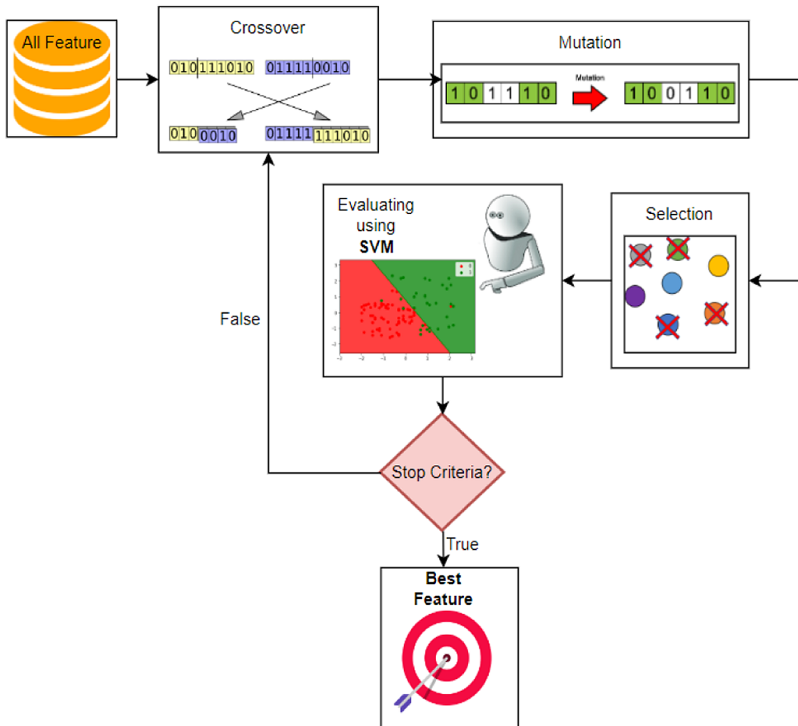
Figure 2 Illustration of the feature selection process of GA-SVM
