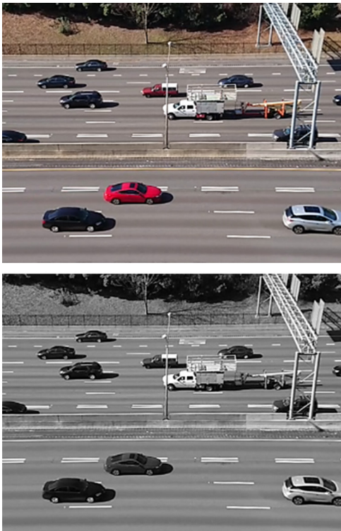
Figure 3 RGB to grayscale conversion of the raw input frame
