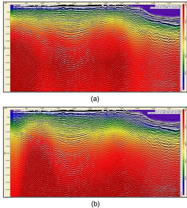
show that the defined SOVI model can accurately pick the time-velocity function that follows the geology of the data. The intelligent prediction results are not very different from that of manual picking. These seismic images have consistent structural information.
