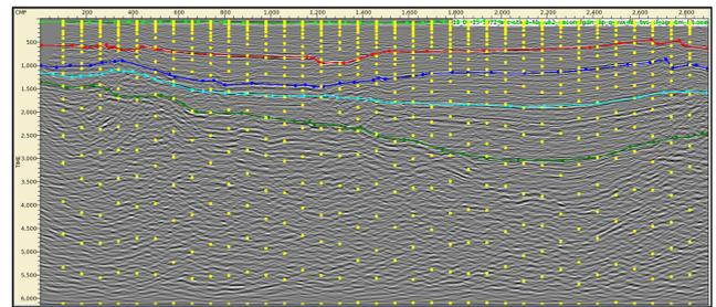
The manually picked velocities and structures of 2D were used as seed points after repositioning them into the defined 3D grid and then into fully populated grid points of 3D volume of velocity and horizons for all the dataset under consideration.
