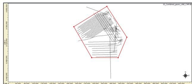
The data beyond the polygon were removed from the study because this extension is a representation of only a 2D dataset in the absence of more seismic lines (Figure 3).
