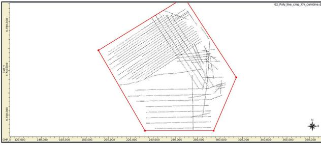
200 m × 200 m cells. This means the final 2D velocity volume will have a velocity location at every 200 m in each direction (North, South, East, and West). The 3D grid definition also converts the X-Y coordinates into an inline-crossline (inline – xline) defined grid. Figure 4 shows an example of a 3D grid of 200 m × 200 m with defined inline-crossline and their X-Y coordinates.
