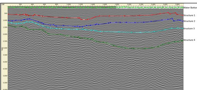
guide the velocity interpolation within a line. It is important to have important structures defined, this will help even if the seismic data do not have a high resolution, then having these horizons for all the lines would help in stabilizing the velocity prediction across the area.
