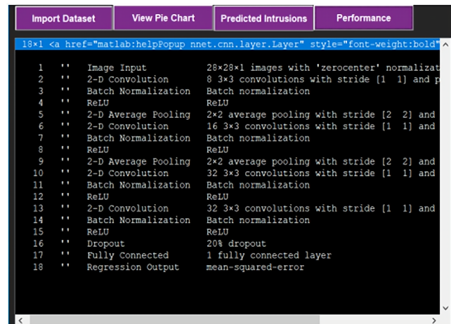
Figure 7 Descriptive representation of layers of CNN model from image dataset
