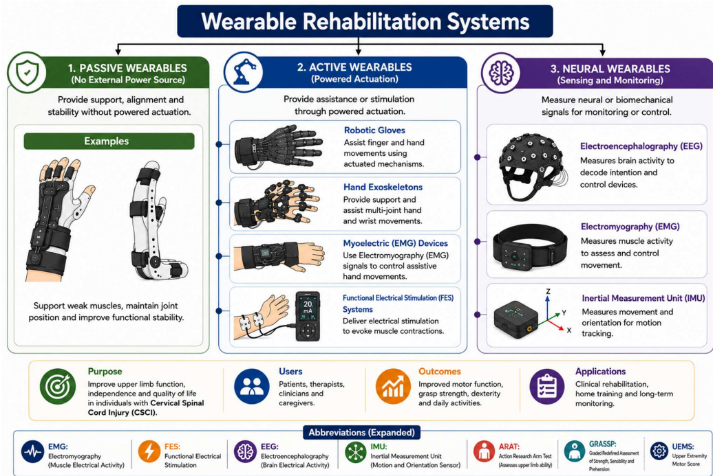
Figure 1 Classification of wearable rehabilitation systems for upper-limb recovery following cervical spinal cord injury. Wearable technologies are categorized into passive wearables, active wearables, and neural wearables according to their primary function. Representative examples, clinical applications, and commonly reported functional outcome measures are summarized
