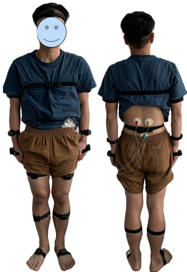
Figure 1 Photo of the experimental participant wearing IMU sensors and a dual-channel sEMG sensor
