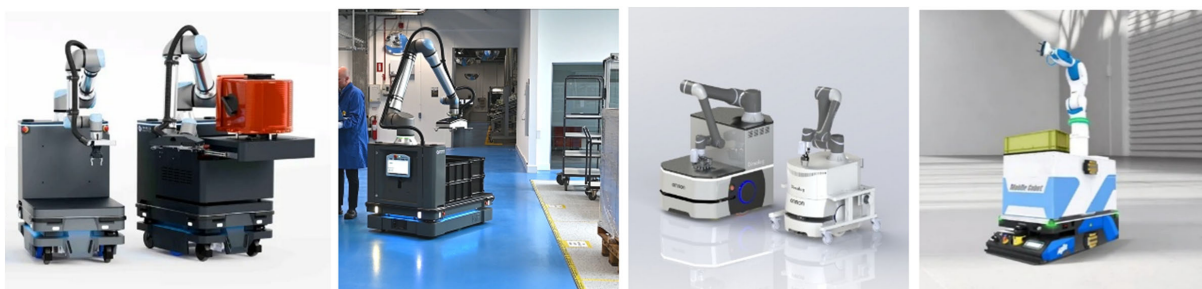
Figure 4 Design variations of collaborative robots on mobile platforms for predictive maintenance applications
