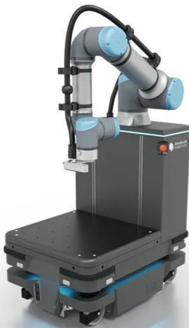
Figure 7 Autonomous mobile robot and collaborative robot equipped with multiple sensors
