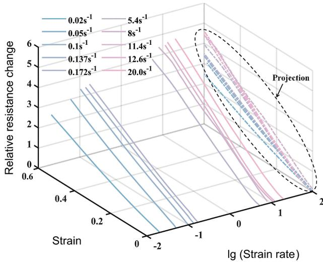
and Cao et al. [18]. By analyzing the strain-relative resistance curves for each experimental run, the sensor specimens' strain-relative resistance behavior was plotted against strain rate, as illustrated in Figure 12.
