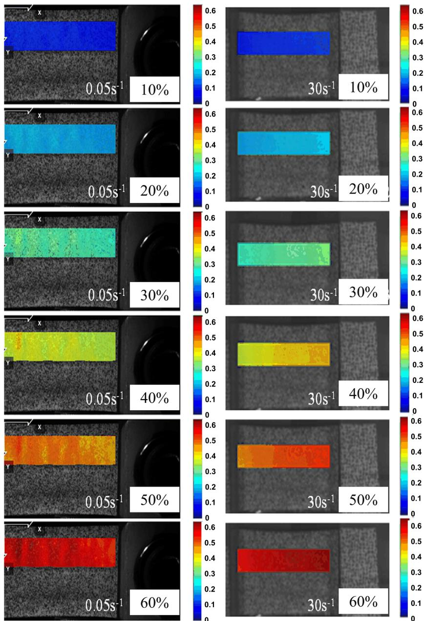
printed fabric sensors [26], where the sensors are claimed to exhibit grid patterns associated with the interaction between the screen-printing process and the fabric structure. In contrast, when the loading rate fell within the dynamic tensile range (at a loading rate of  $30\text{ s}^{-1}$ ), a pronounced gradient trend became evident in the strain field distribution of the sensor.
