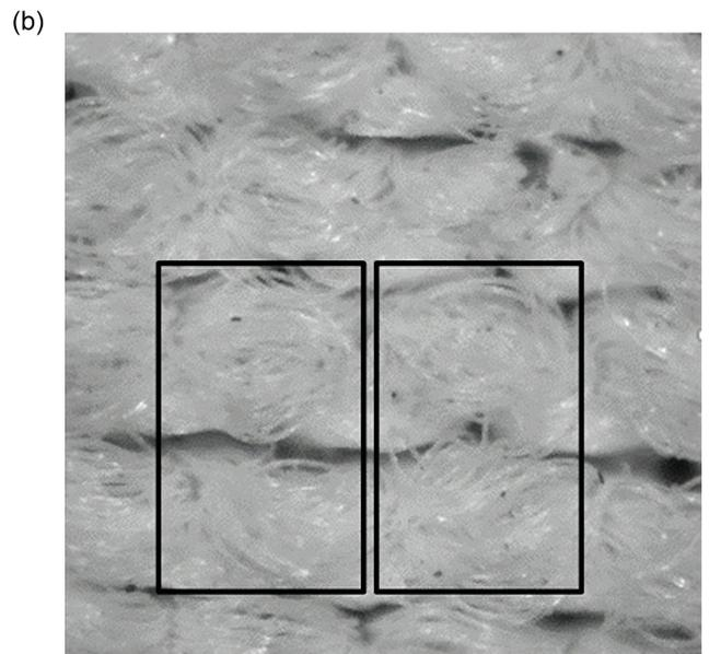
knitting unit network, as depicted in Figure 13 [30]. During stretching, a strain gradient distribution became apparent, with higher strains observed at the edge regions of these unit grids. As the strain intensifies, the strain level disparities within each unit grid become increasingly pronounced.
