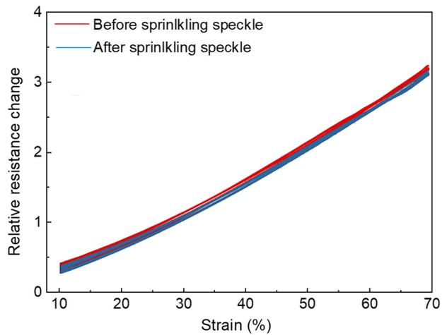
remained largely unchanged post-treatment, the unloading phase was impacted, leading to reduced hysteresis during cyclic stretching. Additionally, the applied speckles' diameter, ranging from 0.5 to 3 mm and differing by an order of magnitude from the specimen size, enables measurement of the continuous strain field in fabric sensors.
