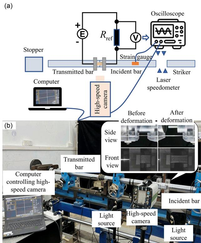
designed fixture. The SHPB's transmission rod facilitates the rapid displacement of one end of the specimen, enabling dynamic tensile loading over time. The specimen is securely fastened to the rod via the fixture, which retains both ends of the specimen on the
