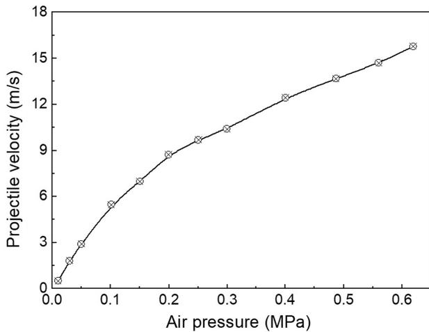
and the incident bar come to a halt, transferring all their kinetic energy to the transmission bar. This causes the transmission bar to move, with its velocity representing the loading velocity applied to the experimental specimen. Calculations show that the Hopkinson bar can theoretically provide loading velocities ranging from 1.2 m/s to 6 m/s, allowing for strain rates ranging from  $20 \text{ s}^{-1}$  to  $120 \text{ s}^{-1}$  to the resistive FSS specimens used in this study.
