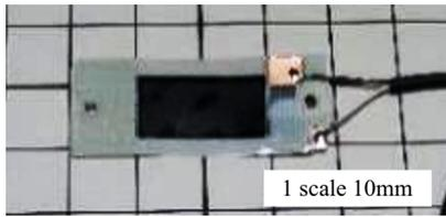
Figure 8 shows the prototype of the DE strain sensor (DESS) using the HNBR. The basic configuration is the same as the DESP described in Figure 7. However, in consideration of attaching it to a robot hand, the shape is a rectangle 10 mm in length and 20 mm in width, and no support material is used.
