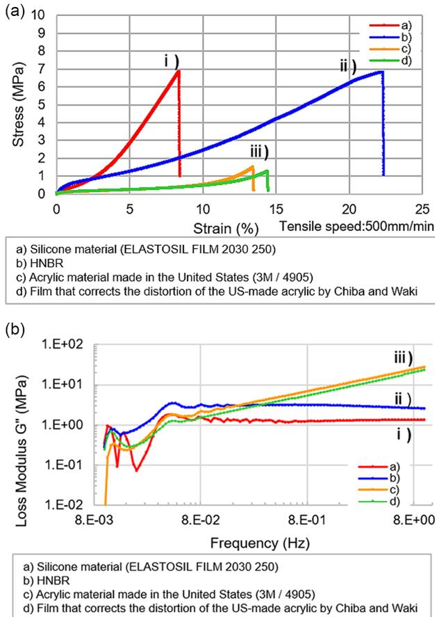
paper, the acrylic elastomer is a commercially available thin sheet (3M 4905). The silicone film is also commercially available, and silicone ELASTOSIL film/2030-250 is used. The HNBR is made by Zeon Corporation and is rolled to a thickness of 200  $\mu\text{m}$ .
