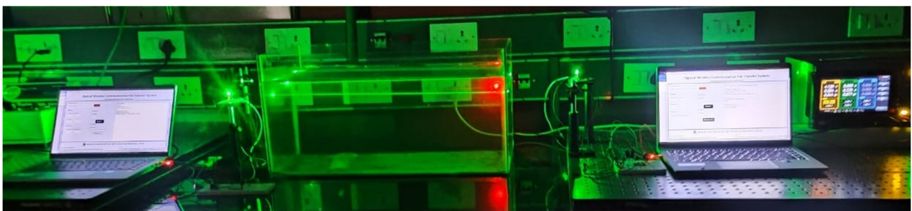
Figure 4 Working setup of underwater optical wireless communication testbed for physical modeling studies
