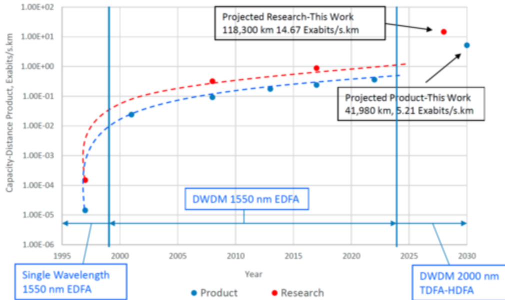
Figure 13 Historical and projected trends for unregenerated subsea lightwave transmission through a single one-core optical fiber in terms of capacity-distance product in Exabits/s.km.
