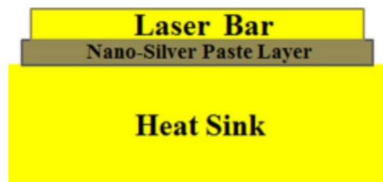
Figure 12 Detailed view of the solder layer of a 60w 808nm CS-Mount laser diode encapsulated with silver Nano-Paste
