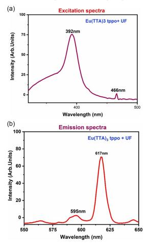
transition, respectively, when excited at 391 nm (Figure 8(b)) [24, 25]. A noteworthy point here is its unique lasing wavelengths as that of the pure pigment. However, the decrease in the emission intensity is loud and vivid.
