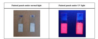
Thickness of the epoxy and UF-based painted panels was determined with the help of wedge shape thin film experiment and was found to be 0.112 and 0.110 cm, respectively. Our previous reports reveal that the pigment, when solvated in toluene for  $10^{-3}$ M, peaked at 258 to 259 nm and 356 to 358 nm that can be allocated to  $\pi \rightarrow \pi^*$  and  $n \rightarrow \pi^*$  optical transitions, and the energy band gap was found to be 3.13 eV [20] and hence not reported here.
