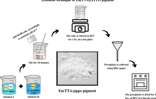
Figure 1 Synthesis technique of Eu(TTA)<sub>3</sub>TPPO pigment Figure 2 Pigment beneath normal daylight and ultraviolet radiation (280–320 nm)
