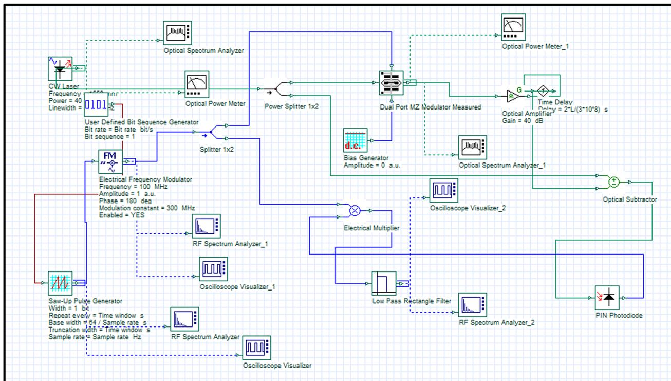
40 dB erbium-doped fiber amplifier. A time delay is introduced in the signal chain, and a reference signal is extracted from the lower arm of the optical power splitter for optical subtraction in the photonic down-conversion process. The optical-to-electrical conversion is performed using a PIN photodiode whose responsivity is 1 A/W.
