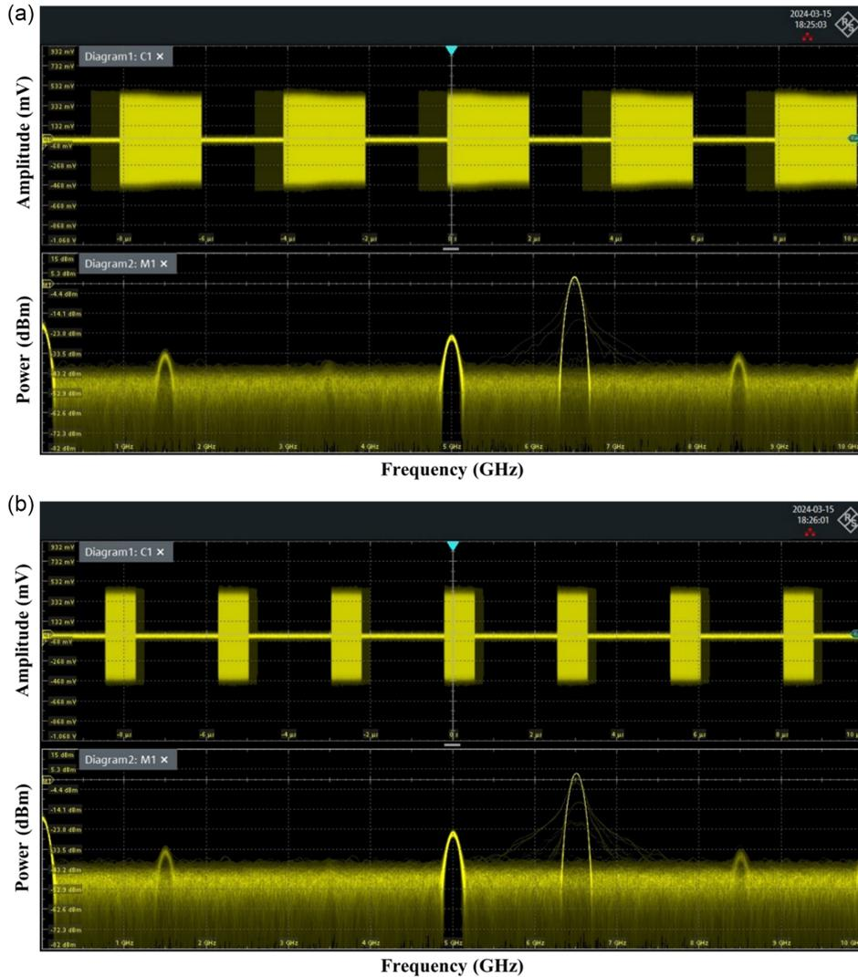
i.e., T-F images. In the RF CW mode, the radar system transmitted a DC-biased multicomponent RF signal whose frequencies are 2 GHz, 5 GHz, 7 GHz, and 8 GHz. The results of our PEWS captured temporal and its spectral signatures are shown in Figure 7(a). As therein, the time domain representation of the captured RF signal has multicomponent which are clearly detectable in the generated spectral profile of the same CW signal.
