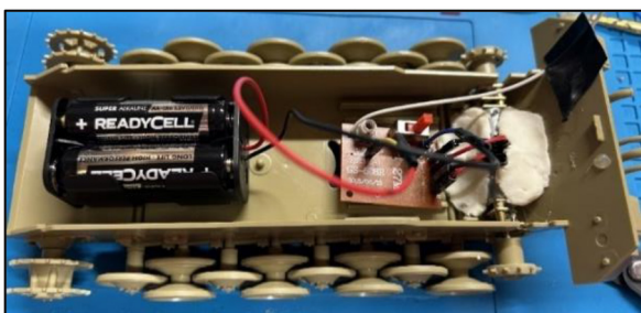
Figure 9 The 6-V N20 motor test
