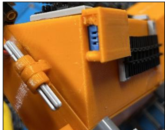
Figure 26 The DHT 11 sensor as it was embedded within the UGV
