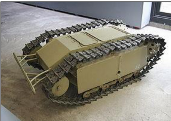
Figure 3 A battery-powered Goliath tracked mine [5]
