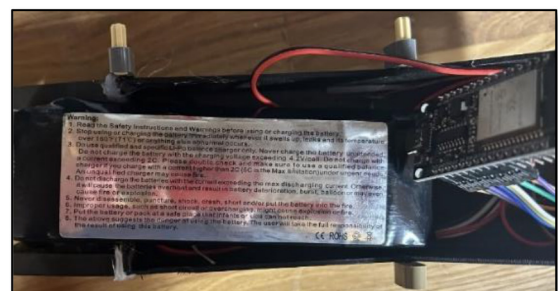
Figure 22 The 3S Li-Po battery in the improved rhomboidal design (in order to accommodate it, a section of the rear hull was removed)
