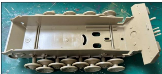
Figure 5 Tamiya's 1990 re-release RC panther tank hull with the motor cutouts visible at the rear
