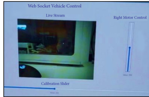
Figure 25 The video streaming running on the UGV
