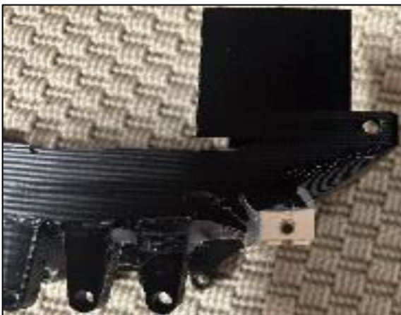
Figure 19 LEGO Technic brick used to mitigate printing failure
