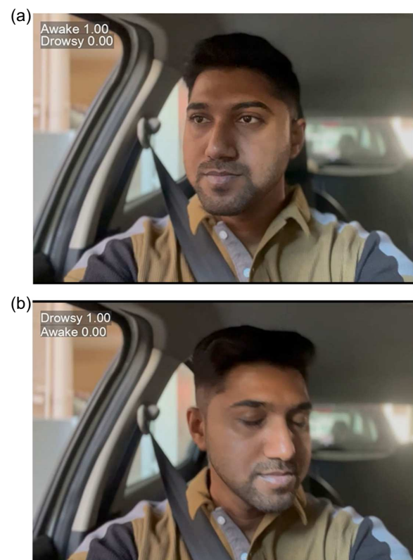
Figure 3 Frame-wise classification using the proposed YOLOv11 model on real-time video streams for drowsiness detection
