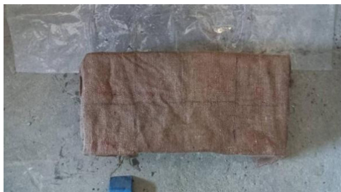
Figure 2 Curing of the samples in air
