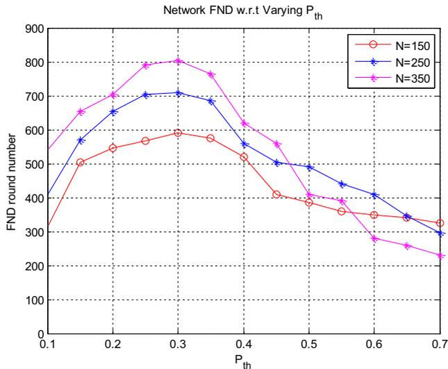
CH's standard and keep communication overheads within the permitted range, a lower value of  $P_{th}$  is suitable for densely deployed node networks. In Figure 6, the higher values of  $P_{th}$  reduce the life of the network sharply in the densely deployed network because of massive communication overheads. As obtained from Figure 6, beyond  $P_{th} = 0.3$ , the network operational life declines quickly. The value of  $P_{th}$  is considered as 0.3 for the suggested network setup.
