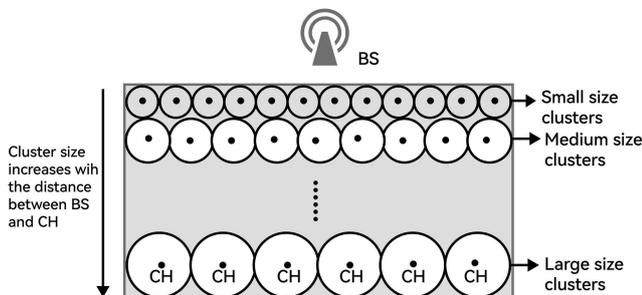
The cluster size relies on the CH to BS distance. The smaller size clusters are near to BS and have lower number of CMs in the particular cluster that reduces the intra-cluster traffic cost. There is less energy consumption by smaller clusters during intra-cluster
