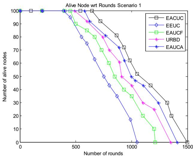
situated in the middle of the monitoring area. Figure 10 designates the alive nodes w.r.t communication rounds for suggested EACUC, EAUCA, URBD, EEUC, and EAUCF protocols. To recapitulate the simulation results, the communication round in which FND and HND as shown in Figure 10 are signposted in Table 3. The first sensor node entirely exhausts its energy at communication rounds 626, 561, 509, 478, and 428, for suggested EACUC, EAUCA, URBD, EAUCF, and EEUC, respectively.
