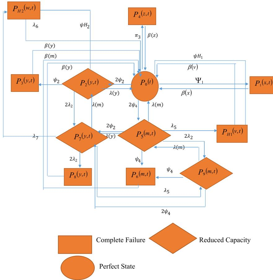
$$\left[ \frac{\partial}{\partial t} + \psi_1 + 2\psi_1 + \psi_3 + 2\psi_4 + \psi_{H1} + \psi_{H1} \right] P_0(t) = \int_0^\infty \beta(x) P_1(x, t) dx + \int_0^\infty \lambda(y) P_2(y, t) dy + \int_0^\infty \beta(z) P_4(z, t) dz + \int_0^\infty \lambda(m) P_5(m, t) dm + \int_0^\infty \beta(v) P_{H1}(v, t) dv + \int_0^\infty \beta(w) P_{H2}(w, t) dw \quad (1)$$
