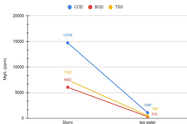
Figure 3 Decreased levels of COD, BOD, and TSS from FDE after being treated into tea water
