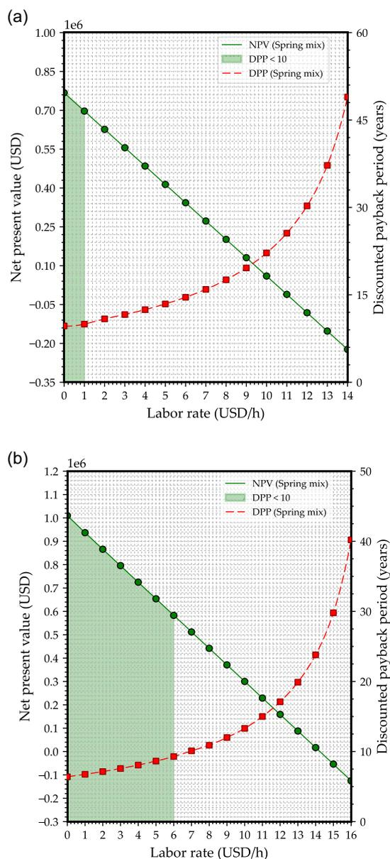
USD/h with the minimum possible CapEx of \$481,800 USD, as shown in Figure 6(b). While ROI is a simple method of profitability calculation, IRR is a more complex calculation that considers the time value of money. Therefore, the labor rate thresholds, below which the IRR values are higher than 10%, are < \$1 USD/h and < \$7 USD/h, respectively, in the base and best cases. These ranges are reasonably close to the thresholds corresponding to the DPP of less than 10 years in Figure 5.
