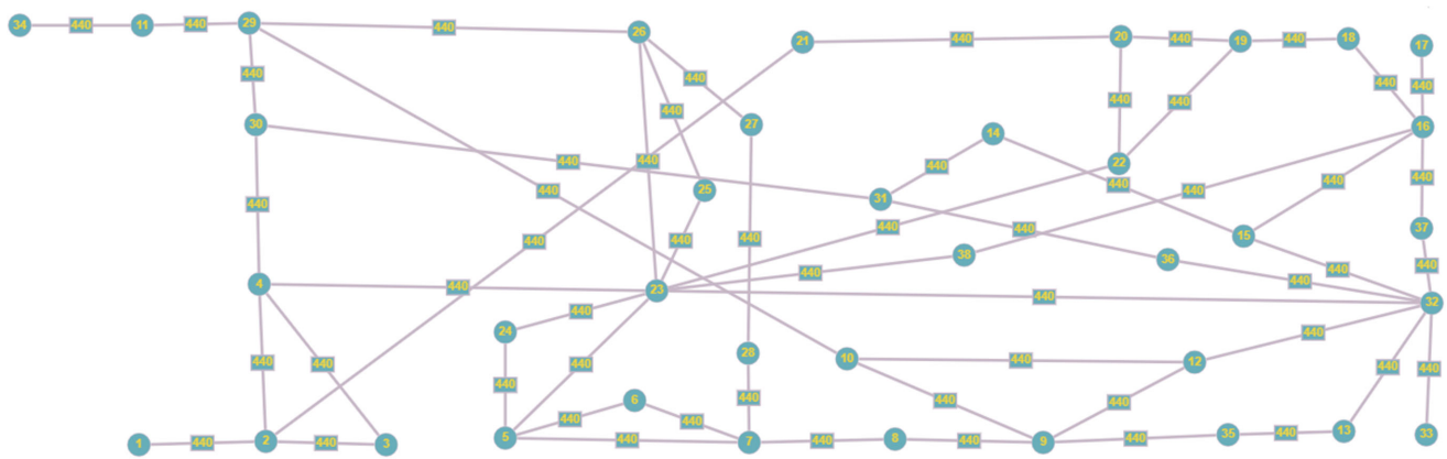
Figure 4 Transmission lines with 440 kV in Brazilian territory, belonging only to the state of São Paulo
