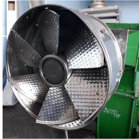
Figure 1 Air distributor with twisting plates for a swirled air jet
