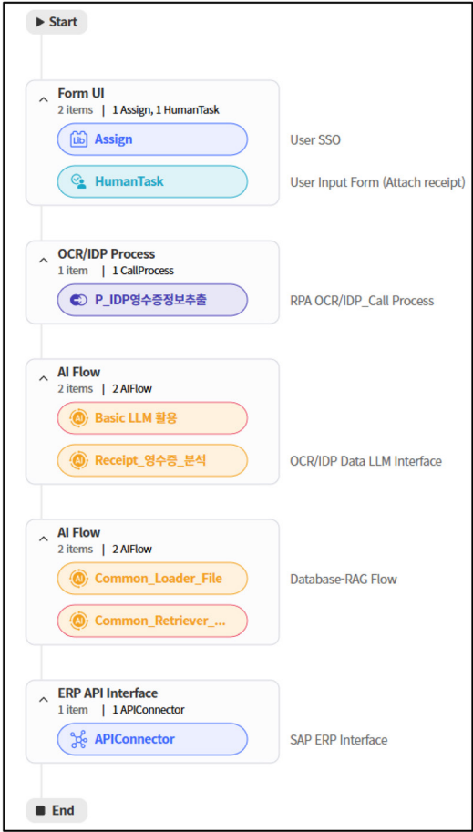
Figure 19 Human task and overall workflow integration process flow
