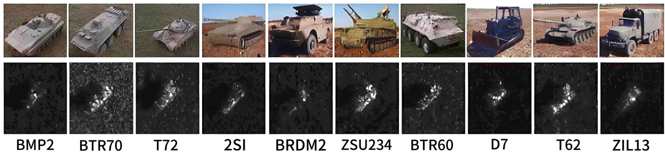
Figure 2 Ten kinds of items from the MSTAR dataset are represented by optical images and associated SAR images Source [17]
