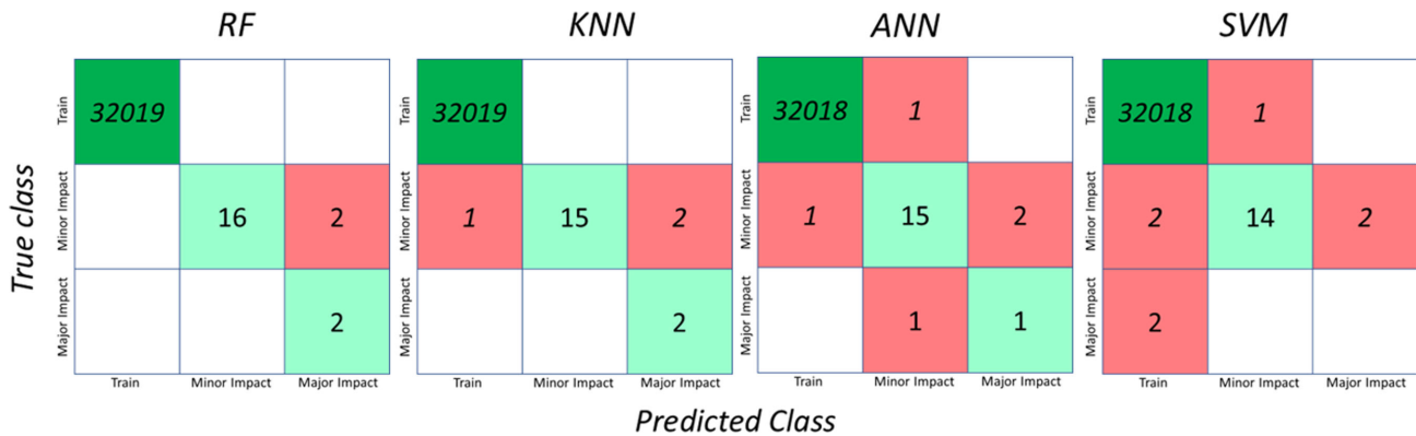
Figure 13 Confusion matrices obtained using the tested data for RF, KNN, ANN, and SVM models, from left to right
