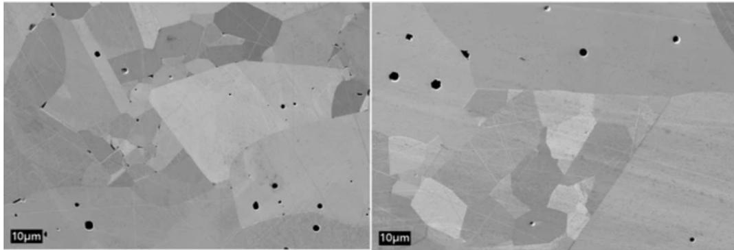
sample was mechanically ground with SiC paper before polishing with diamond suspensions of varying grain sizes (15, 3, 1, 0.1 µm). The WC tasters were mechanically slurped. The samples were cleaned with deionised water and degreased with ethanol before testing. The electrolyte was a 1 M NaOH solution comprised of sodium hydroxide pellets p.a. (Carl Roth) and deionised water.
