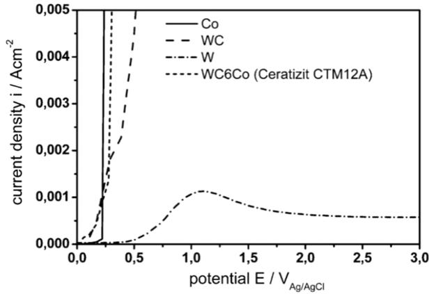
polishing techniques. Figures 4 and 5 (Lohrengel et al., 2014) depict cyclovoltammograms of cobalt and electropolished tungsten wires, pure WC, then saleable WC/Co examples in the aqueous solution of NaNO<sub>3</sub>, and Figure 6 (Lohrengel et al., 2014) is about investigations on the current transients of a 5 s potentiostat, pure WC in aqueous sodium chloride. Figure 7 (Lohrengel et al., 2014) depicts the microstructure. The grains of WC are soft grey. WC grain breaches
