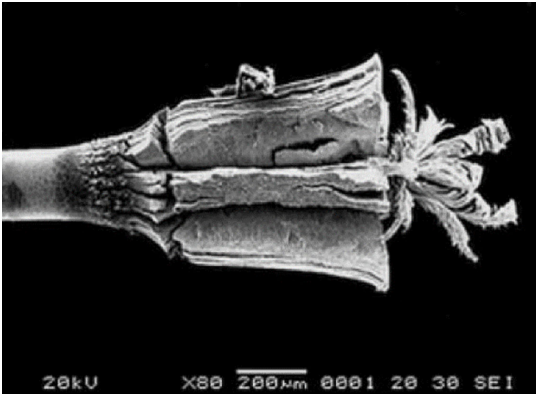
Figure 23 Sludge accumulation on the sample during the etching of WC
