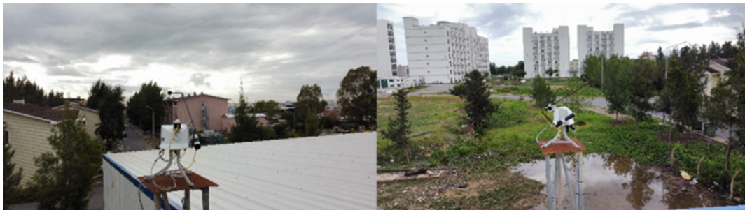
Figure 7 The integrated data logger, RAZON + , has two intelligent irradiance sensors: a shaded pyranometer for measuring DHI and a pyrheliometer for measuring DNI
