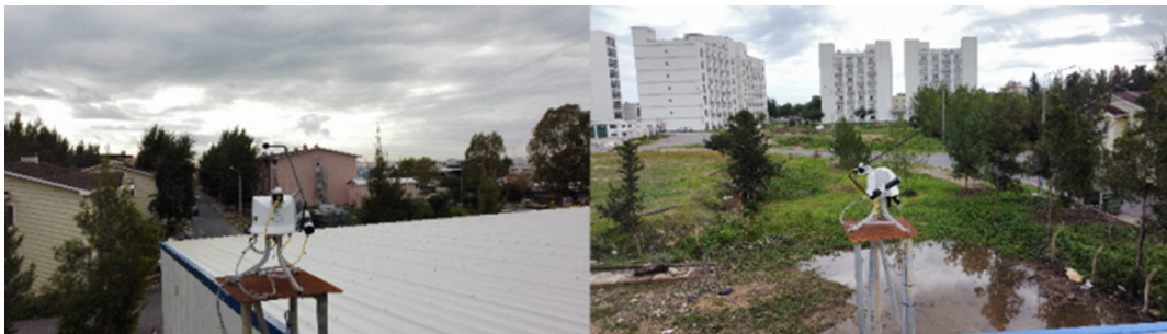
Figure 7 The integrated data logger, RAZON+, has two intelligent irradiance sensors: a shaded pyranometer for measuring DHI and a pyrhelimeter for measuring DNI
