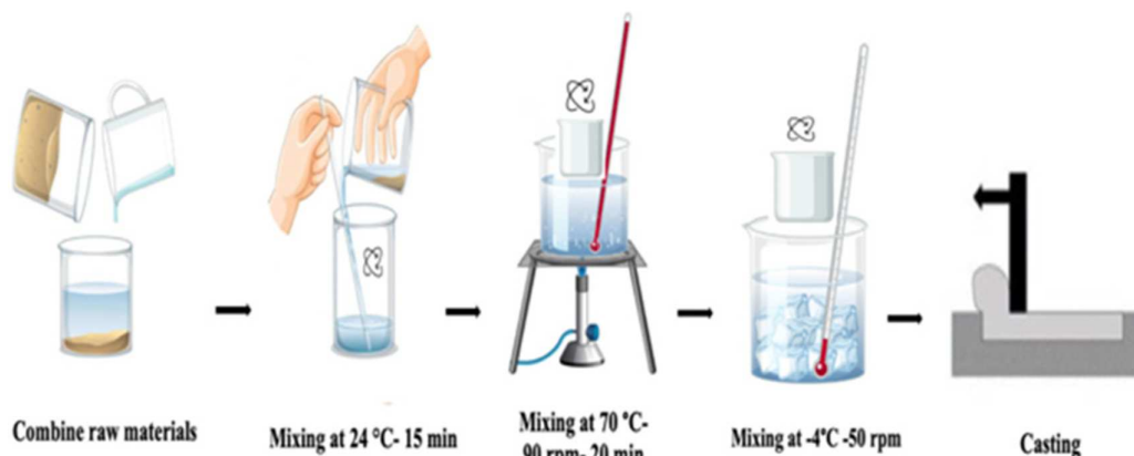
Figure 2 The fabrication process of composites
