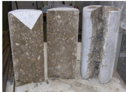
Figure 21 Spilling strength for plain and fiber concrete
