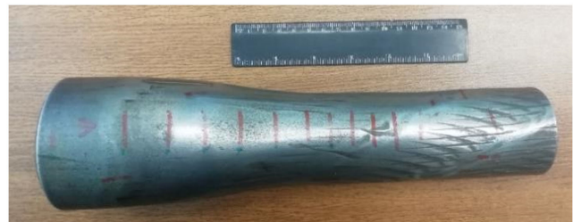
Figure 4 A sample of a forged tube of two different cross-sections for comparison before and after the radial forging process. The tube shows the sections required for hardness testing
