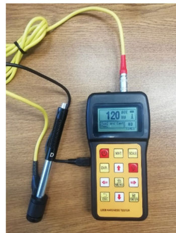
Figure 5 Hardness tester with impact device type D and connecting cable
