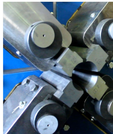
Figure 7 Radial forging machine with a feeding system during the practical test
