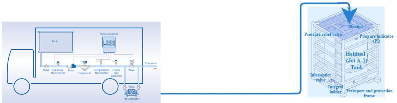
Figure 4 Process flow diagram for the inside of the Jet A-1 tanker
