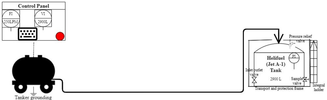
Figure 3 Filling and storage process flow chart of Jet A-1 from tanker to tank in CLS
