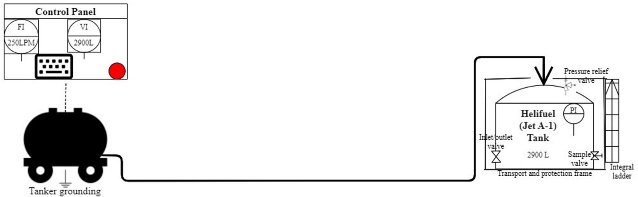
Figure 3 Filling and storage process flow chart of Jet A-1 from tanker to tank in CLS
