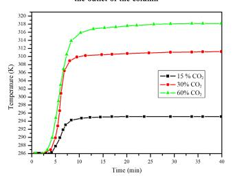
concentration given at the beginning of adsorption (<<20 min), when the temperature increment gradient is higher. The temperature gradient hits the established stage when the adsorption time exceeds 20 min, where further changes are comparatively small in comparison with adsorption time. This is a result of adsorbent bed's  $CO_2$  saturation.
