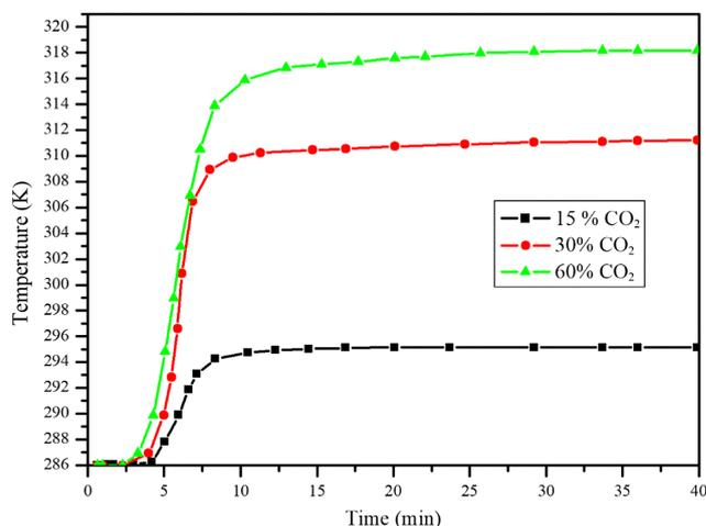
concentration given at the beginning of adsorption ( $\ll 20$  min), when the temperature increment gradient is higher. The temperature gradient hits the established stage when the adsorption time exceeds 20 min, where further changes are comparatively small in comparison with adsorption time. This is a result of adsorbent bed's  $\text{CO}_2$  saturation.
