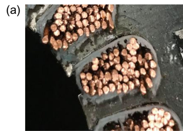
Sectioned stator coil
