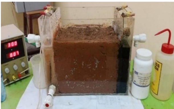
Filter media-enhanced EKR of COCS
