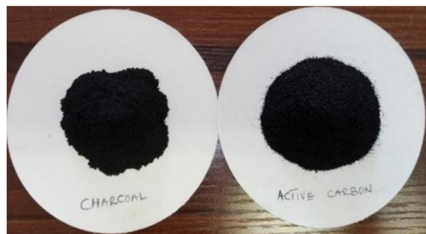
Figure 1 Charcoal and active carbon filter media materials
