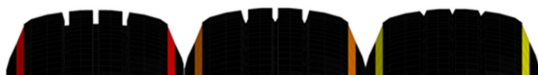
Figure 7 FEA tire wear simulation setup for 100%, 50%, and 25% groove depth truck tires (Ly & El-Sayegh, 2022)
